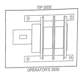
The bottom of the winch drum is 70cm above the foundation
